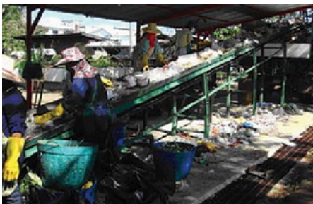
Conveyer Belt for Manual Separation of Waste
